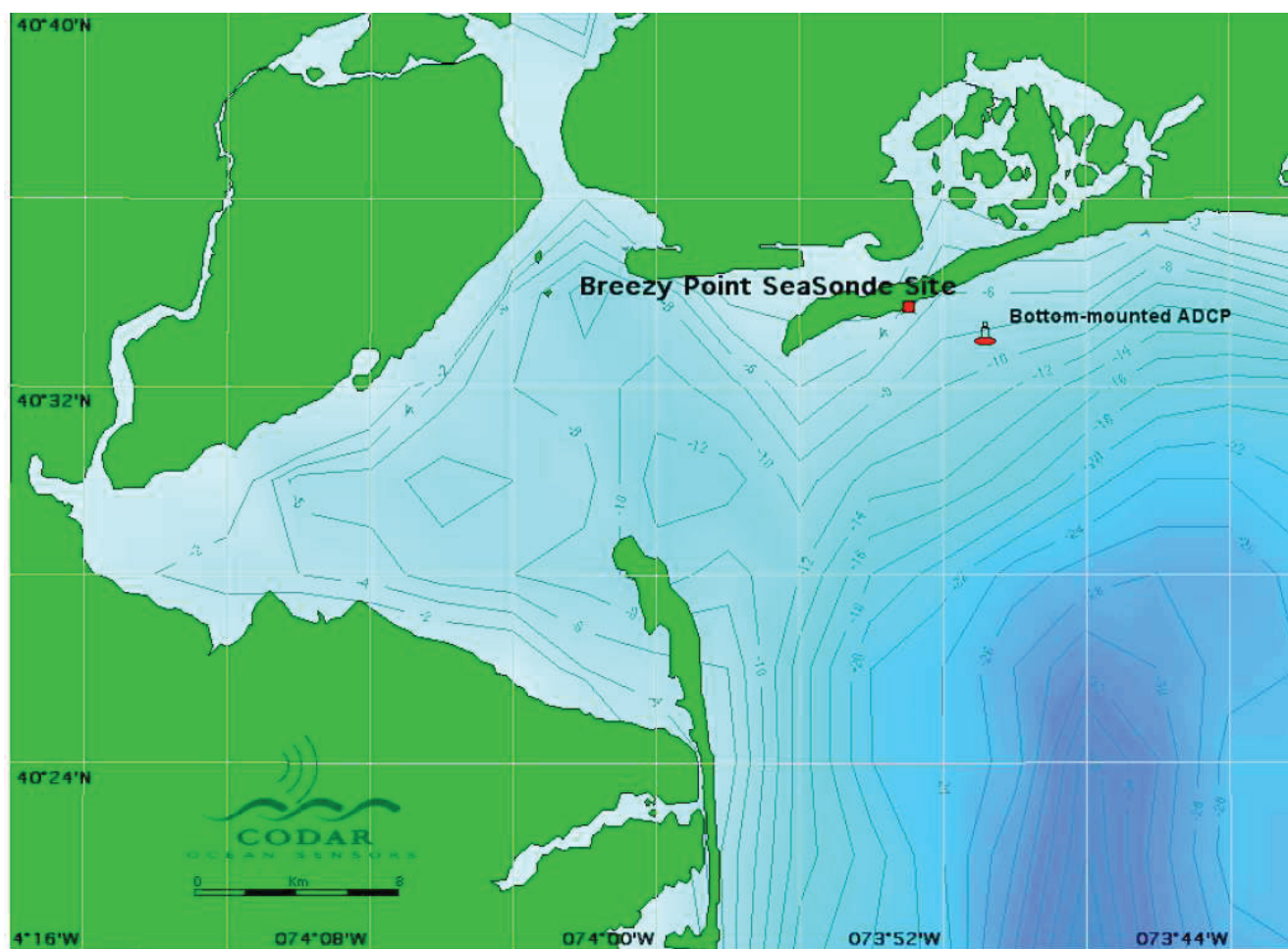
Figure 12. The coastline and bathymetry (contours in meters) around Breezy Point, New Jersey, showing the positions of the SeaSonde and the bottom-mounted ADCP.
