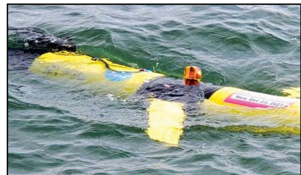
Glider RU34 has a passive acoustic monitor mounted top to listen for underwater sounds.
