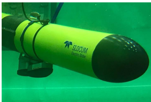
Figure 1. Front end of a Slocum glider with integrated multi-frequency AZFP echosounder (38, 125, and 200 kHz transducers). The AZFP transducers are oriented 22.5 degrees from glider axis to omit pings directly downward.
