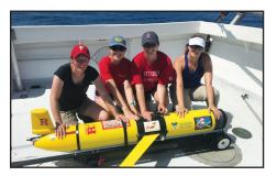
RUCOOL deployed the first glider with integrated pH sensor for observations of ocean acidification in coastal ocean systems, demonstrating the ability for gliders to routinely provide high resolution water column data that can be applied to OA monitoring efforts on regional and national scales through glider networks.
