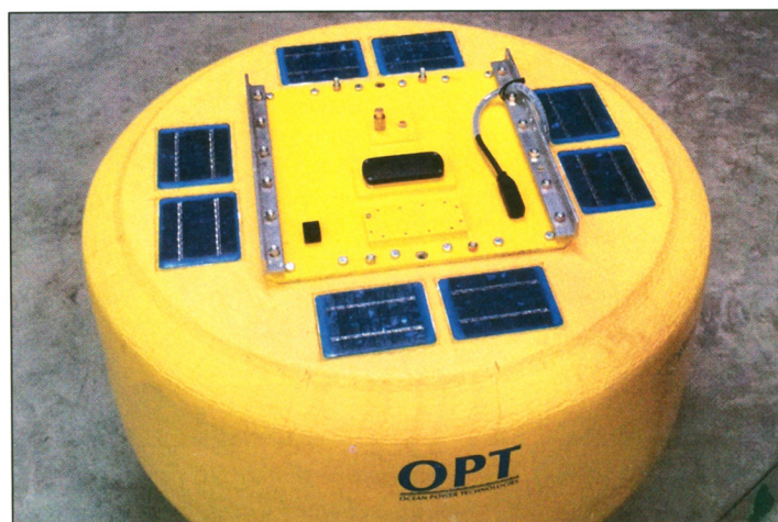
Figure 5 Communications relay buoy - the Micro-Buoy
