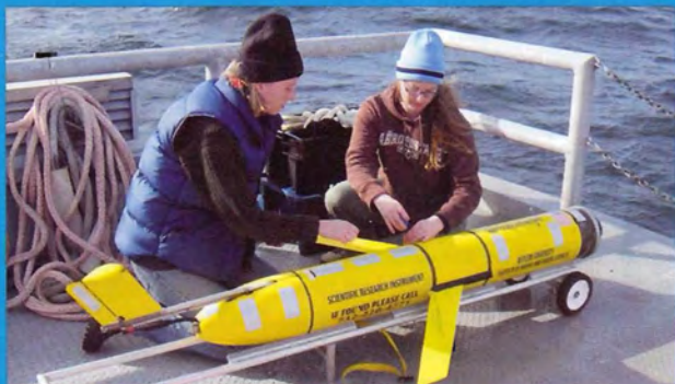
Jennifer Bosch (left), a research scientist at RUCOOL, and Naomi Flemming, an oceanography graduate student at Rutgers, prepare a Slocum Glider for deployment into the Atlantic Ocean aboard a towboat from Sea Tow Atlantic City (N.J.).
