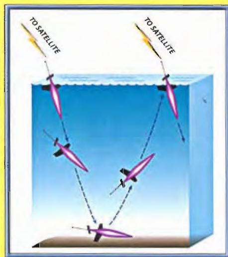
Slocum Glider "swims" in saw-tooth pattern
