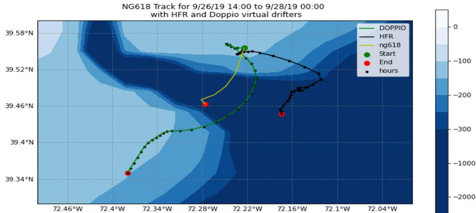
Figure 1: OpenDrift virtual drifter simulation covering the period of 9/26/2019 14:00 UTC to 9/28/2019 00:00 UTC. Actual glider track in yellow, Doppio virtual drifter in green, and HFR virtual drifter in black. Each simulation was started at the green point, the red points mark each end of track, and the black points signify each virtual drifter data point which are one hour apart.
