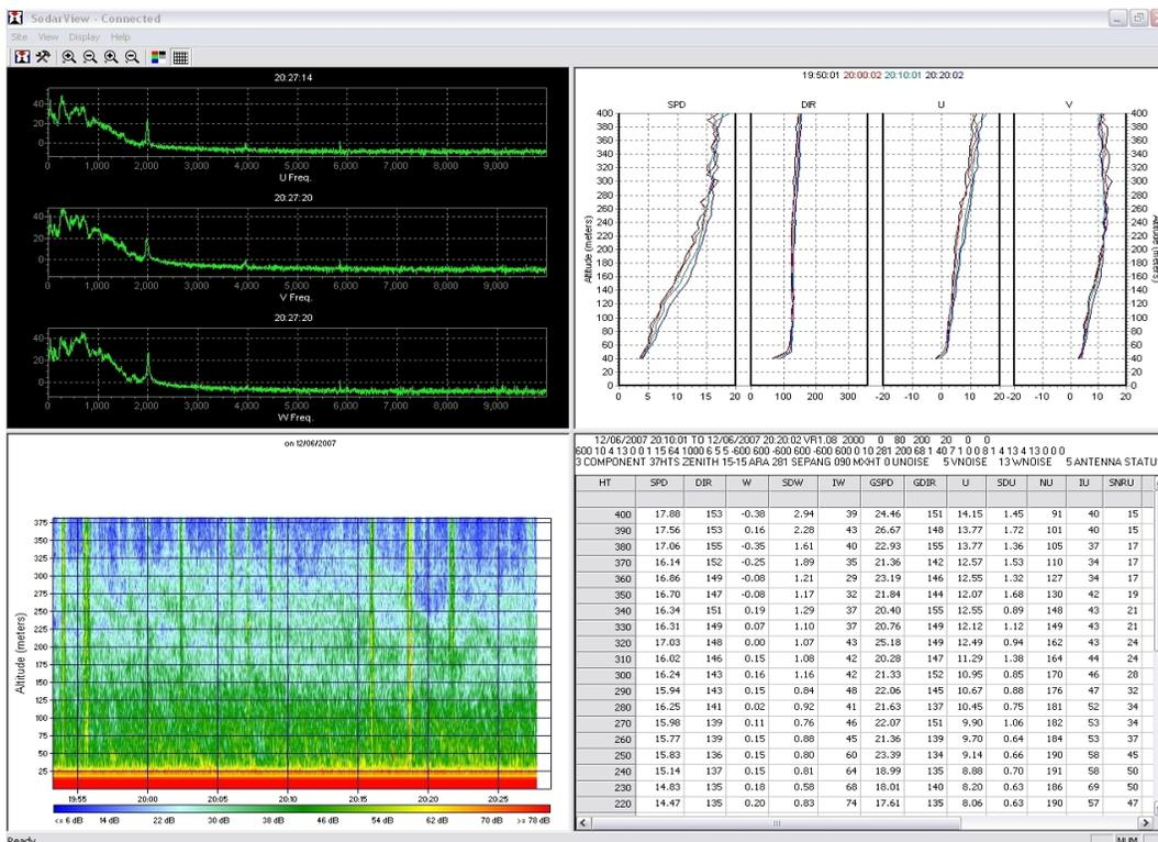
Example SODAR Data Output Showing Wind Velocity Profiles that extend from ~40m to > 200m
