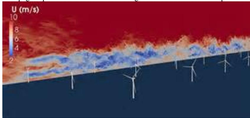
**Simulation of turbulent wake effects among several WTGs located within a large OSW facility.**
