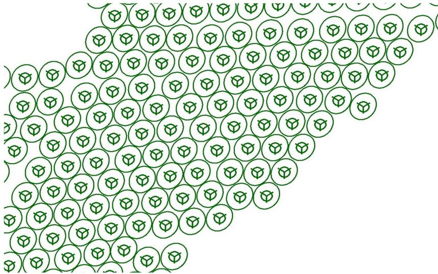
**Hypothetical WTG Array showing 10D X12D spacing with a “staggered” configuration to account for prevailing winds along with the effects of local wind flow patterns (e.g., the sea breeze circulation).**
