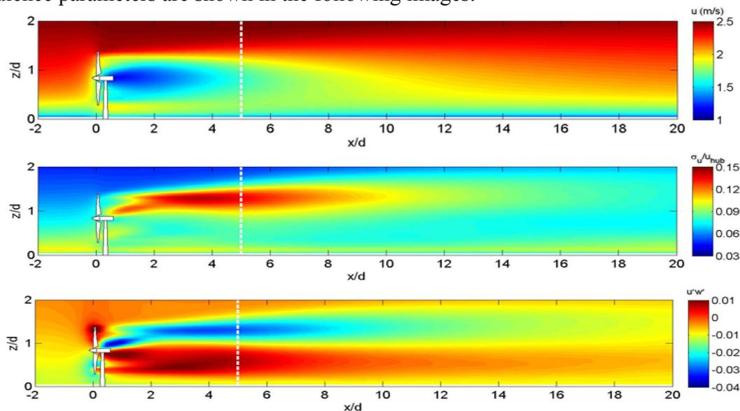
Simulation results for turbulence parameters obtained using LES with a Lagrangian scale-dependent dynamic model: average velocity (top), turbulence intensity (middle), kinematic shear stress (bottom).
