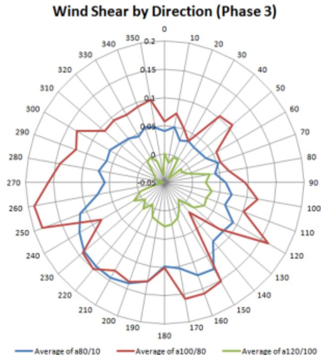
The data presented in the preceding graphic provide pertinent information regarding offshore wind shear characteristics that are associated with WTG dimensions (i.e., hub and blade tip heights). This information is summarized in the below bullet items:
