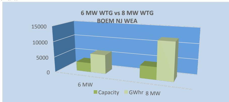
**Comparison of maximum installed capacities (MWs) and resultant annual energy production (GWhr) projected for 6 MW and 8 MW WTGs that could be installed within the BOEM NJ WEA.**
