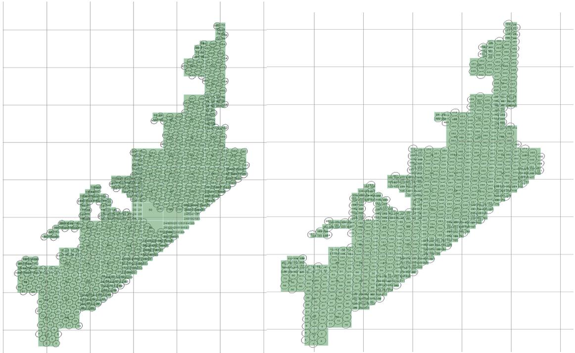
**Maximum BOEM NJ WEA installed Capacity: 3000 MW using 6 MW WTGs; 4000 MW using 8 MW WTGs**
