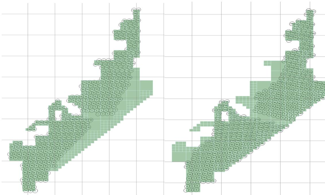
**BOEM NJ WEA installed Capacity (~3000 MW using 8MW WTGs) for respectively the near-shore and farthest offshore locations delineated for the BOEM NJ WEA.**
