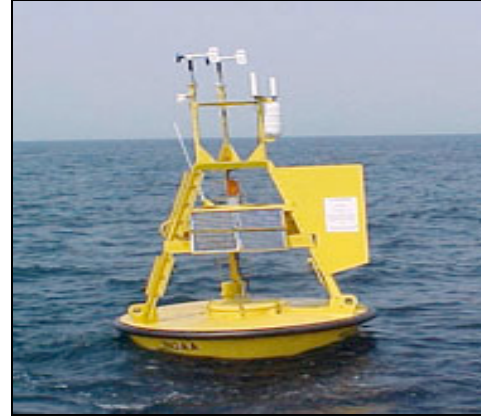
Figure 10: NOAA Monitoring Buoy (Anemometer Height at 5m Above MSL)
