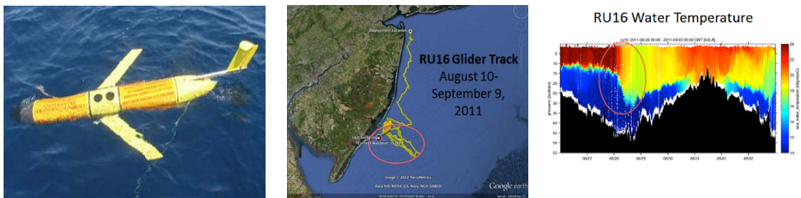
Figure 66: RU-16 Glider Deployed During Hurricane Irene, Glider Track, and Monitored Ocean Temps
