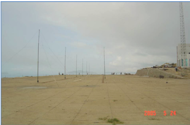
Fig. 3.2. The receiving array of the Dongshan OSMAR station
