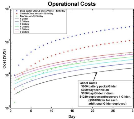
Figure 2. The costs in United States dollars for maintaining ships and gliders at sea. Ship costs represent the average daily charge that varies with ship class based on averages in the year 2005. The glider costs include the expenses of deploying, maintaining, and recovering a glider.
