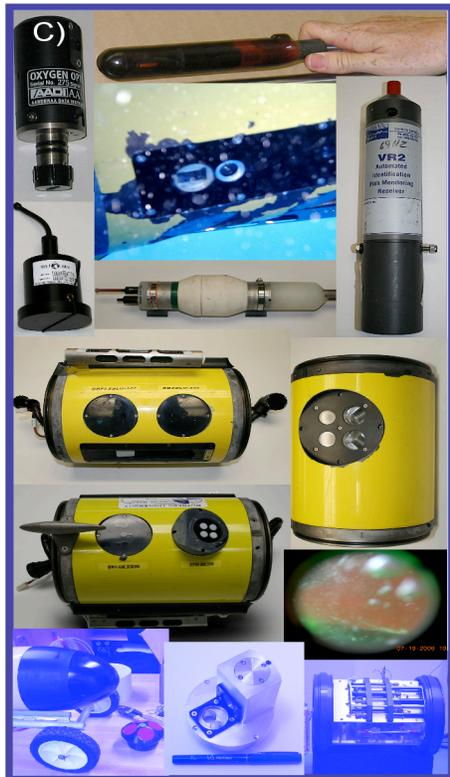
Figure 5. The sensors that have been carried on Webb gliders. They include (starting at the top left panel) oxygen, passive acoustic, attenuation, chlorophyll/colored dissolved organic fluorimeters, turbulence, fish finders, scattering and backscattering packages, spectral backscatter, radiometer, digital cameras, acoustic doppler measurements, fast repetition rate fluorometry, and absorption.
