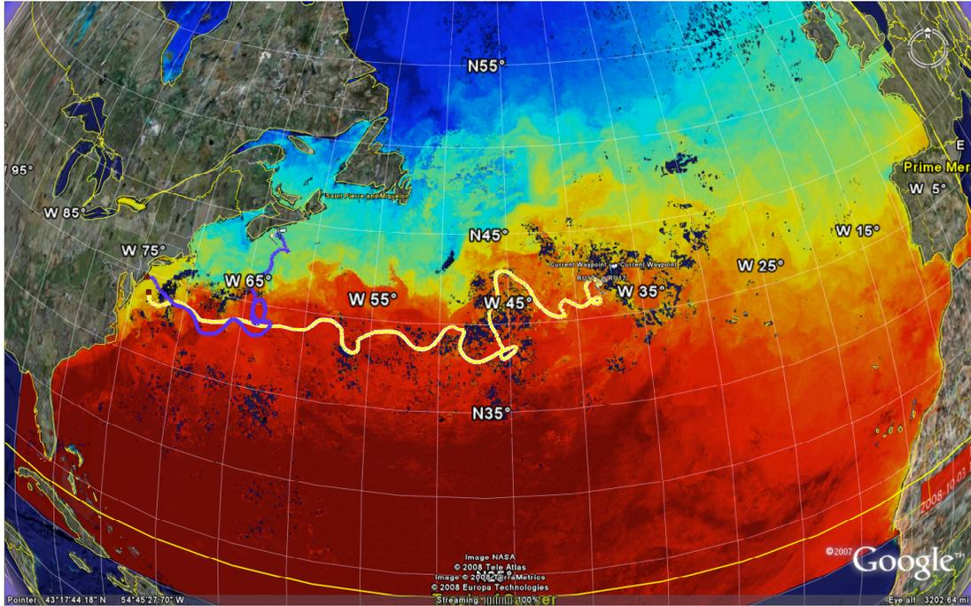
Figure 7. The path of undergraduate glider missions focused on long duration missions. The blue line shows the successful flight from New Jersey to Halifax. The yellow line shows the student's first attempt to cross the Atlantic.
