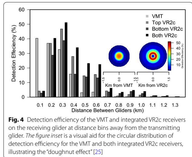
**Fig. 4** Detection efficiency of the VMT and integrated VR2c receivers on the receiving glider at distance bins away from the transmitting glider. The figure inset is a visual aid for the circular distribution of detection efficiency for the VMT and both integrated VR2c receivers, illustrating the “doughnut effect” [25]
