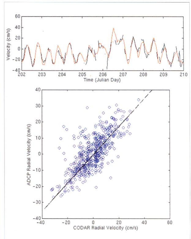
Figure 3: Raw data comparisons between South-site SeaSonde and ADCP bin at 4.5 m depth. Lower is scatter plot for month of July (6.7 cm/s rms difference); upper is one-week time series
