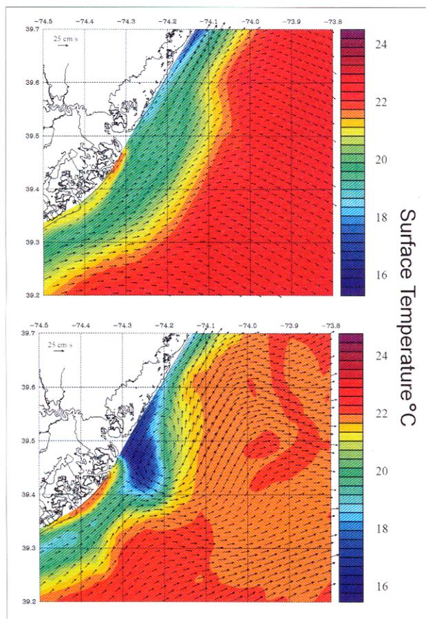
Figure 2: Ocean model outputs for July 17, 1998 both with (lower) and without (upper) SeaSonde data assimilation. Model fails to predict observed eddy without SeaSonde input
