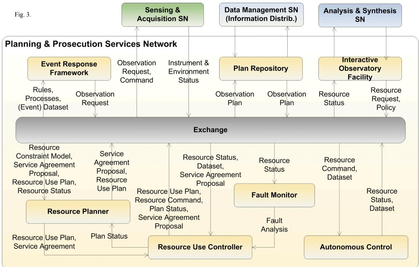
The *Fault Monitor* is a separate component analyzing and overseeing resource status, providing fault analysis input to the Resource Use Controller that in turn can revise plans within their local service agreements or return to the Resource Planner for re-planning.
