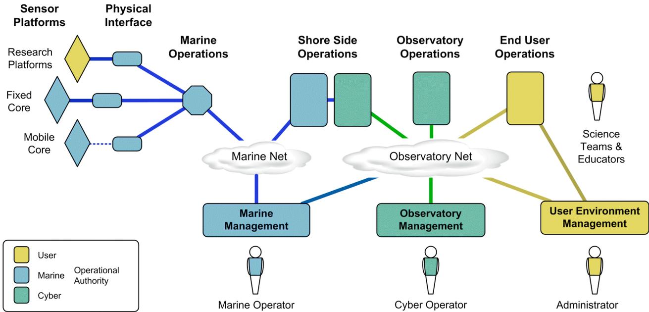
Fig. 3. OOI integrated observatory operational domains
