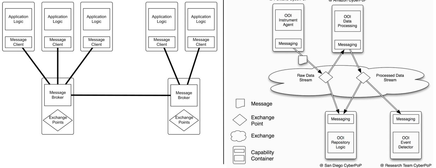
Fig. 3. Message-Broker Architecture and Scenario
