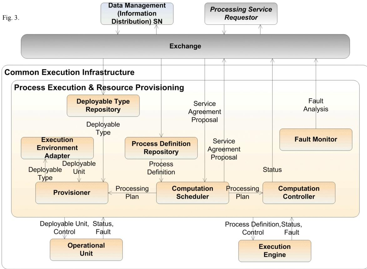
*Controller*. The controller is the entity responsible for enacting the processing plan within the service agreement. It provides status about scheduled and ongoing computations to the Exchange for routing to the service requestor. A *Fault Monitor* is an independent entity monitoring ongoing processes and providing fault analysis information to the service requestor via the Exchange.
