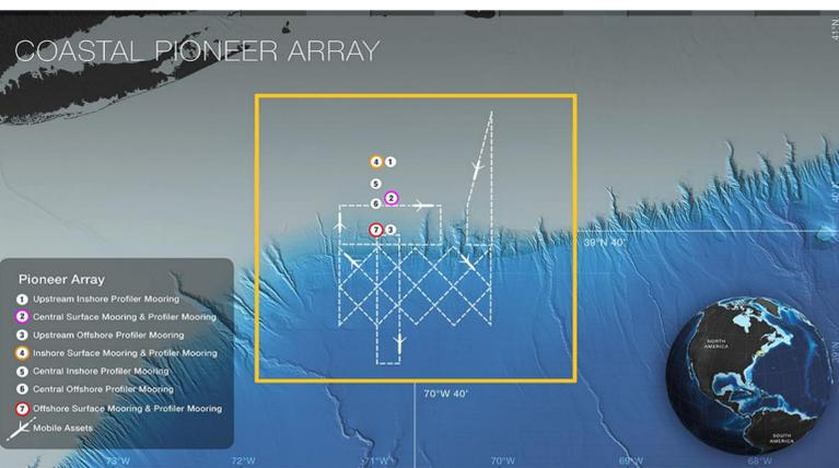
Map displaying the 7 moored locations constituting the Coastal Pioneer Array. Smaller shapes drawn by white marks display coverage area of gliders and Autonomous Underwater Vehicles providing complementary data. This poster focuses on mooring data however the future efforts will use the Slocum glider data. Figure from the Ocean Observatories Initiative.
