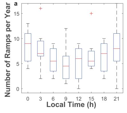
J F M A M J J A S O N D Month Ramp-up events detected using 7 years (2005-2012) of observations from buoy 44009 off the coast of Delaware, with threshold criteria of a ramp being a 50% increase in expected power production over a 1 hour time period. Figure (a) shows the median, range, and first and third quartiles of ramp events detected each year, by hour; and (b) by month.
