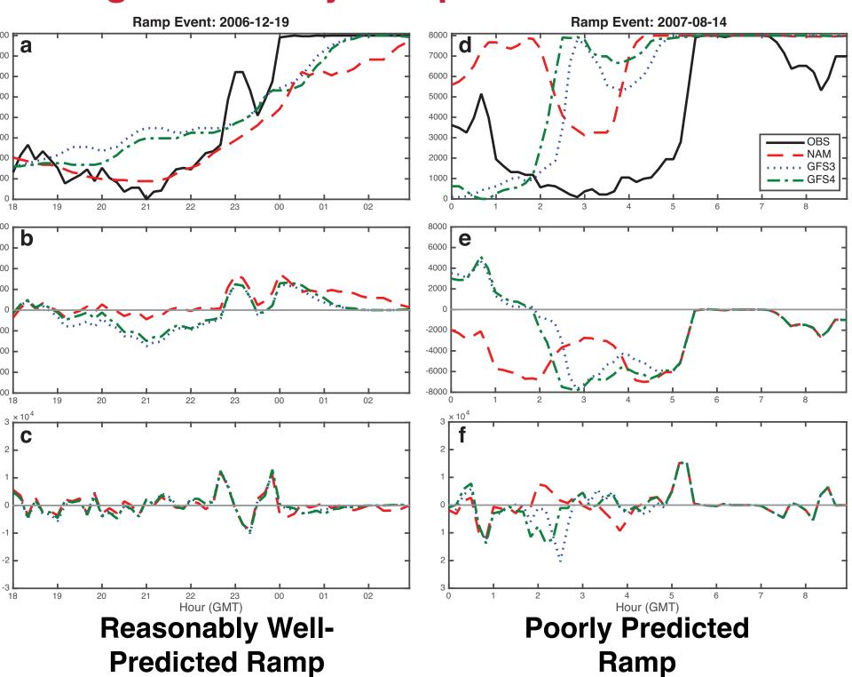
These figures show two example case study ramp-up events, with the observed ramp from observations at 44009 in black, and three different WRF model runs in the colored lines.
