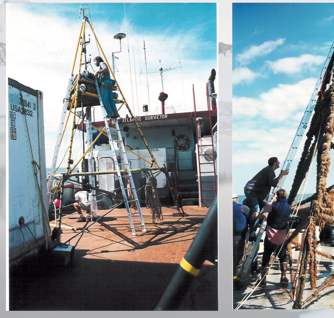
Benthic Acoustic Stress Sensor (BASS) Tripod Before and After Summer Deployment at LEO
