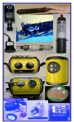
Figure 5. The sensors that have been carried on Webb gliders. They include (starting at the top left panel) oxygen, passive acoustic, attenuation, chlorophyll/colored dissolved organic flourometers, turbulence, fish finders, scattering and backscattering packages, spectral backscatter, radiometer, digital cameras, acoustic doppler measurements, fast repetition rate flourometry, and absorption.
