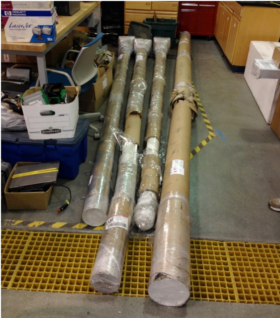
Figure 4: Three receive antenna masts and one 5 MHz transmit antenna.
