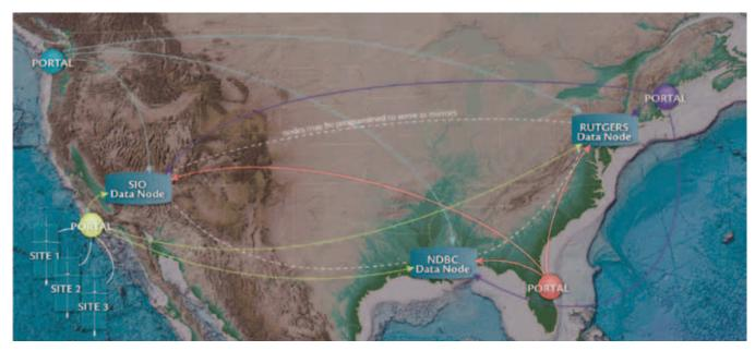
*Figure 4: National Data Nodes and Regional Data Portals, Dotted lines indicate national failover capability. Data flow from four example Portals to the three National Data Nodes are indicated by arrows. As an example, data flow from three HFRs to a Regional Portal (lower left) is also shown.*
