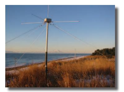
Photo 3: Coastal Ocean Dynamics Applications Radar (CODAR) Receive Antenna (foreground) with Transmit Antenna in background. Cook Inlet, Alaska.
