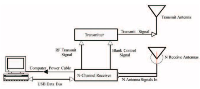
Figure A-2: Diagram of Core HFR Components and Data Flow
