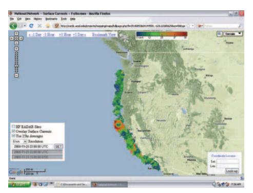
Figure 1: Real-time display from existing west coast HFR network
