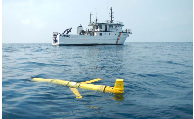
Figure 3: A photograph of RU29, an autonomous underwater glider that successfully crossed the Atlantic Ocean in 2014. Behind RU29, the Oceanographic Research Vessel Alpha Delphini, from the University of São Paulo
