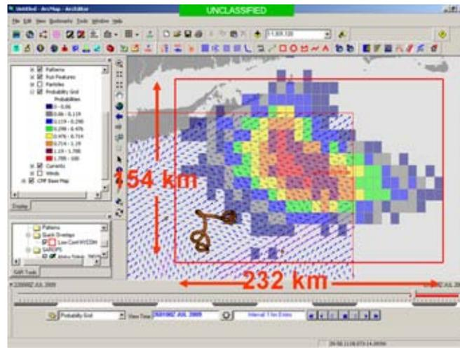
dicted dispersion of the 5000 simulated drifters using the HYCOM data source is shown in Figure 6. The search area using the HYCOM data equates to 36,000 km<sup>2</sup>. The predicted dispersion after 4 days of the 5000 simulated drifters using the HF radar data source is shown in Figure 7. The search area using the HF radar data equates to
