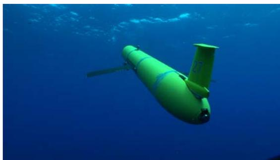
Figure 1: A photograph of RU27, an autonomous underwater glider that successfully crossed the Atlantic Ocean in 2009.
