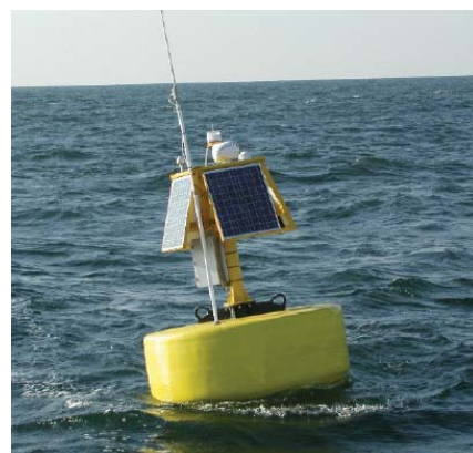
Shore-based CODAR buoy-based bi-static transmitter.
