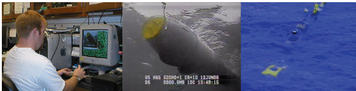
FIG. 4. Remote real-time capture of a REMUS AUV using a Sebotix ROV. Here, all three images were taken simultaneously with (left) the remote operator, (middle) ROV view of the AUV as it approaches for capture (also seen on operators screen in left), and (right) the aerial view of the ROV approaching the AUV. The effort took place on 11 Jun 2006 from the California Polytechnic State University's pier facility in San Luis Obispo Bay, CA.
