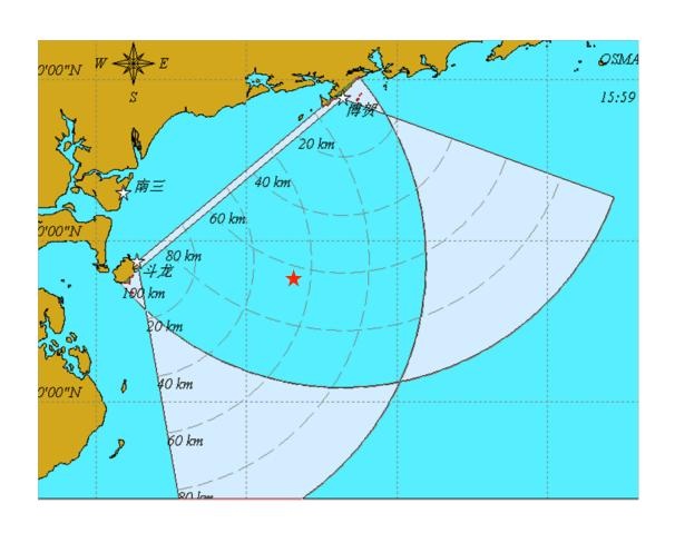
Two HF Radar stations equipped with OSMAR-S100 (developed by Wuhan University), were located in Bohe and Doulong, and established in 2014. their distance is about 100km
